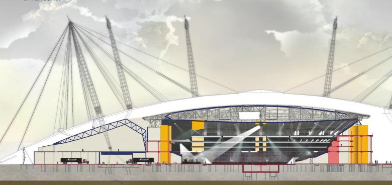
London's new O<sub>2</sub> Arena uses a steel roof, erected with an innovative lifting operation, to top what was designed to be Europe's most acoustically advanced concert venue.
