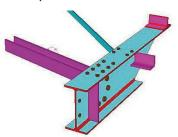
Now you can go directly from a Tekla or X Steel 3-D model into Ficep's proprietary software where we automatically generate the CNC program for not just the holes but also the scribing data for all the required layout locations without any manual programming!
