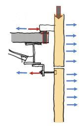
Façade attachments must be designed to resist lateral and gravity loads.
